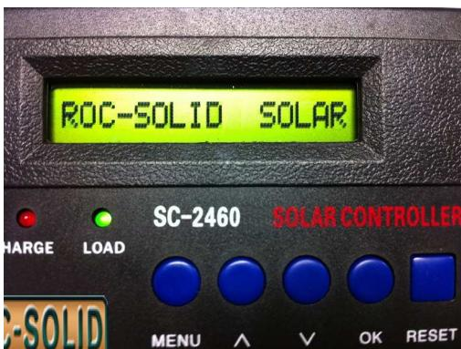
The solar controller has 5 buttons used to select the display mode and modify the default settings to the user requirements.
